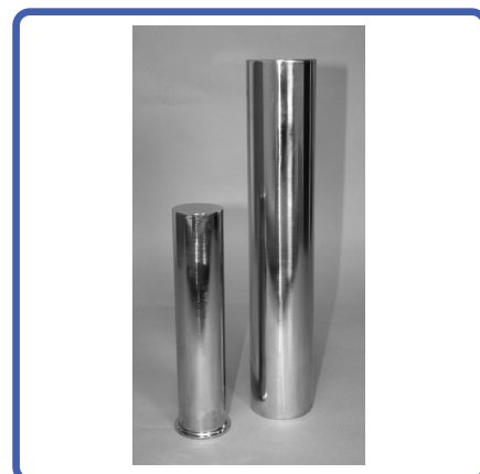
The above picture shows the vacuum shroud and radiation shield for the cryostat.
